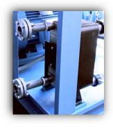
The hydraulic pump is mounted with a bell housing which provides the pump with perfect alignment and facilitates replacement. Pump drive is from a face mounted, fully enclosed, fan-cooled electric motor coupled directly via a flexible drive coupling with replaceable insert spider. The pump drive speed is 1800 RPM at 60 Hz (1500 RPM at 50 Hz).
