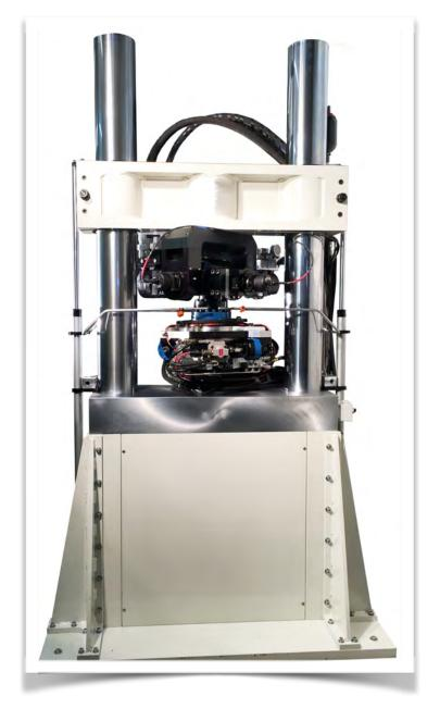
the cocking rotary actuators with angular displacement sensors. An axial torsion actuator package was installed in the base for the other two inputs. The integrated control system is able to resolve all the forces angles and displacements into their constituent inputs to the specimen. Two systems were built with similar specifications. One was designed to run at low frequency for characterization, the other at 22Hz for fatigue testing.
