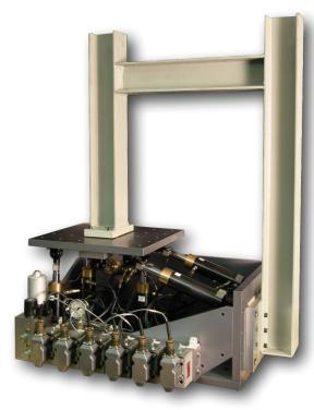
For example, columns can be mounted to the strong floor, with the LBCB on the top, grounded to one of the walls. **Multiple units can be tied together and programmed in one unified plane** using our highly configurable Multi-Degree-of-Freedom (MDoF) control algorithm.
