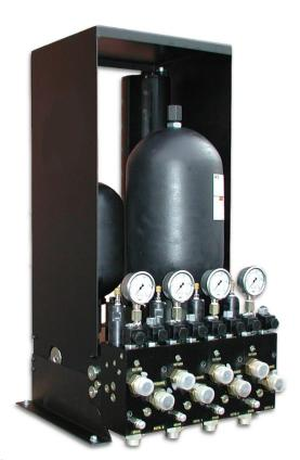
Bia West manifolds have full flow 10 micron filtration for the main circuit, and where applicable, 3 micron full flow filtration for the servo valve pilot and hydrostatic bearing circuits. Fluid
