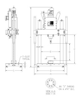
The load cell can be mounted to the actuator piston rod or the platen
